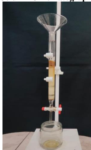
Fig. 7: Column chromatography analysis done to isolate fractions of samples
